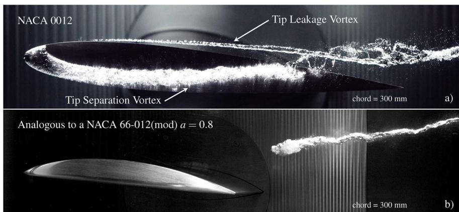
FIG. 1. Cavitation in a tip leakage flow for a truncated “square” edge tip and a tip with a rounded profile: (a) NACA0012 profile for a maximum thickness to gap ratio of  $\tau = 0.16$ ,  $\sigma = 1$ , and  $\alpha = 5^\circ$  and (b) custom profile, analogous to a NACA66-012(mod) thickness profile with a NACA  $a = 0.8$  camber line,  $\sigma = 1$ , and  $\tau = 0.2$ .
